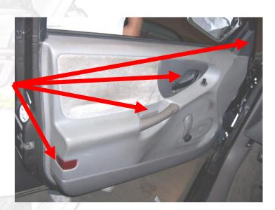
Once all of the screws are removed, detach the trim panel from the door, working around the door with a plastic trim panel tool to disengage the clips, disconnect any electrical connectors and remove the trim panel from the vehicle by lifting it up and away form the door.
