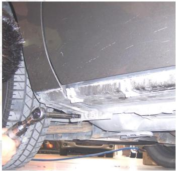
Remove the mounting bolts along the upper edge of the fender and carefully remove the fender.
