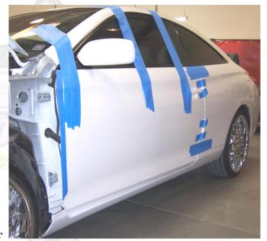
Hint\* Use painter's tape to protect the edges of the fenders and the doors.
