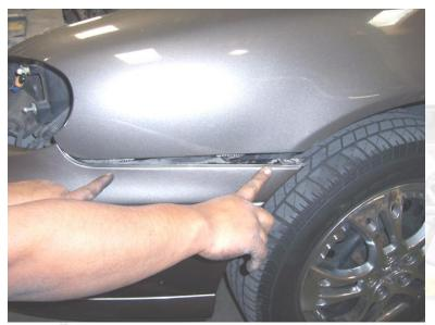
With the headlight removed you will have access to (2) 10mm bolts and (2) plastic clips this will allow you to pull on the bumper and release it from the fender.
